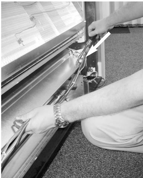
Figure 53: Loosen the four bolts (2 & 2) at either end of the fan board to begin board removal.
