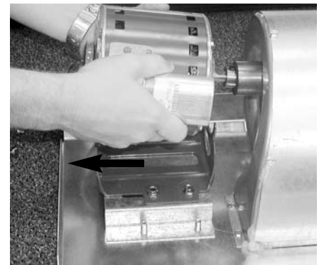
Figure 57: Remove the fan motor by lifting up and pulling forward.
